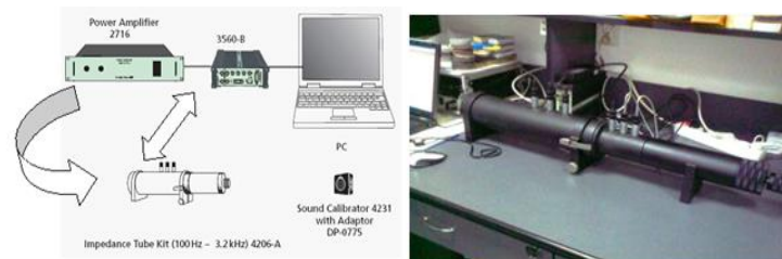
Fig. 2. General scheme of the acoustic interferometer measuring system
